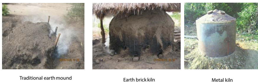
Plate 4: Technologies used for charcoal production in Ghana analyzed
