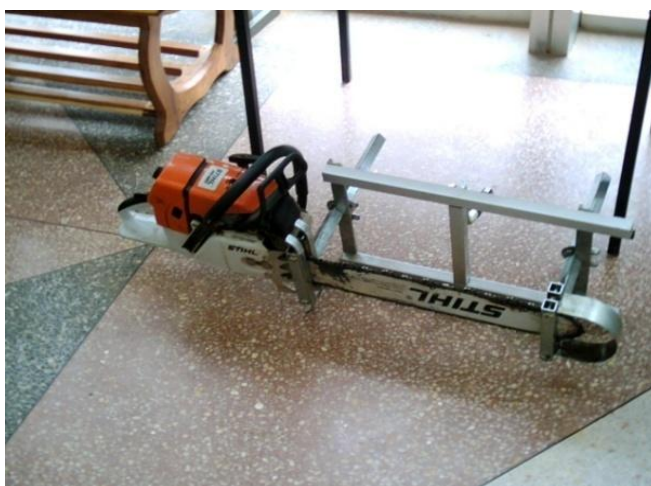
Plate 5 Chainsaw with sawing attachments
